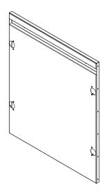
The CLIP standard hinges can be installed on the left or right, depending on which side you want the doors to open.
