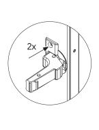
Install the 2 mounting plates, cross using 2 x 2 truss head screws.
