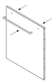
Align the door using the adjusting screws and align the stop with the stopper plates.
